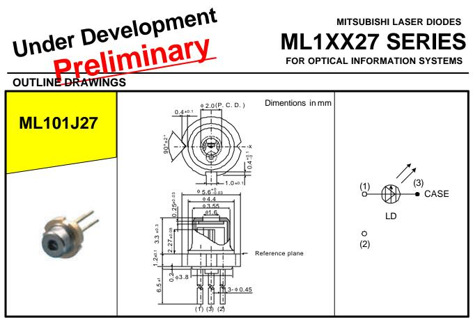
There is no model with a monitor photo diode in ML1XX27 series.
