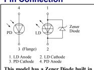
This model has a Zener Diode built in as a protection circuit against static electricity.
