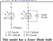
This model has a Zener Diode built in as a protection circuit against
